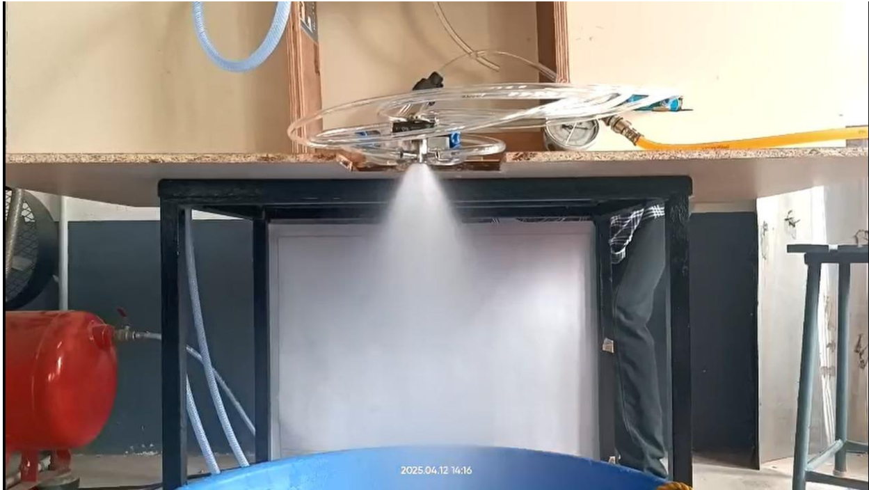
Sample test of the atomization behavior
