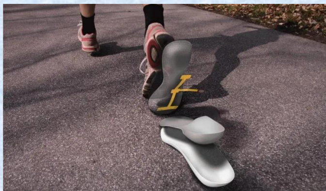
Smart insole with a graphene sensing system that can help detect early signs of foot ulcers before they form. Credit: Bon bouton
