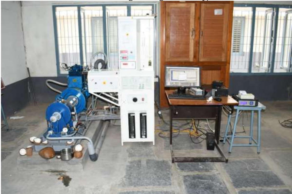
**CRDI Diesel engine with AVL Gas analyzer**
