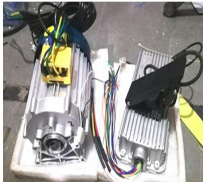
Motor , Controller and Peddle throttle
