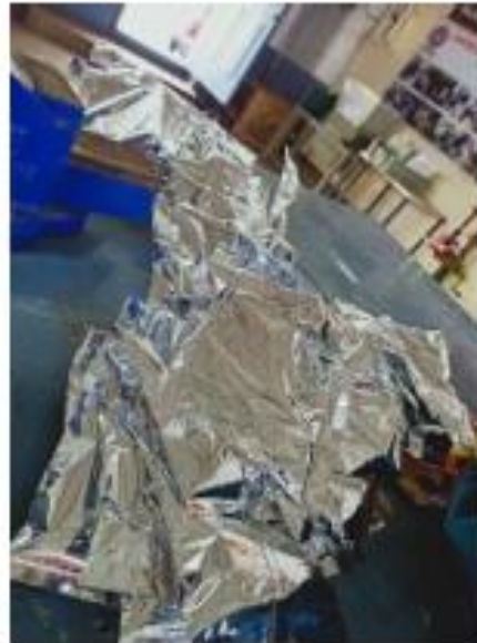
PCM in aluminium packets
