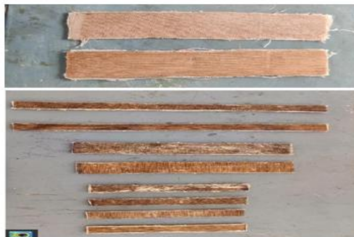
Composites made using hand layup procedure
