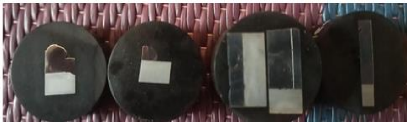
Mounting for the Specimen for testing the hardness and the microstructure
