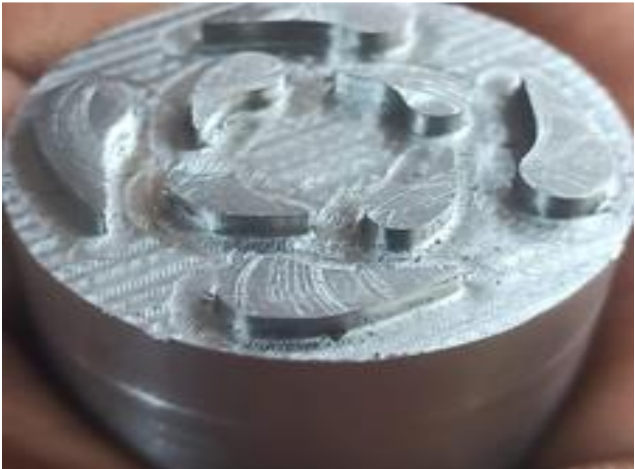
Fabrication of a tool in a CNC with H13 Material
